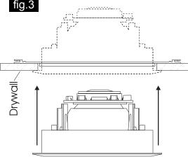
**10.** Attach the metal grille by inserting it into the grooves in the bezel.
